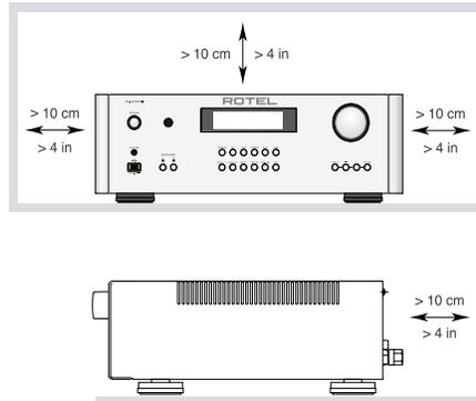
**WARNING:** The rear panel power cord connector is the mains power disconnect device. The device must be located in an open area that allows access to the cord connector.
