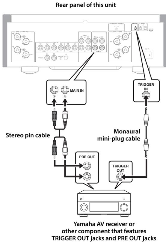
When the power to the connected component is turned on, the power to this unit is also turned on. Simultaneously, the input source to the unit is set to MAIN DIRECT. If MAIN DIRECT has been selected as the input source for this unit, when the power to the connected component is turned off, this unit will enter standby mode.
