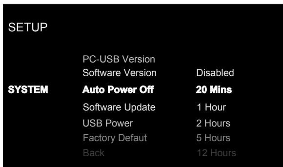
This System menu in the Setup menu, provides the following options, selected by placing the highlight on the desired line using the  $\wedge/\surd$  (D) arrow buttons and pressing the Enter (K) button. This action displays the right side options allowing changes. Change the options using the  $\wedge/\surd$  (D) arrow buttons and press the Enter (K) button to confirm.
