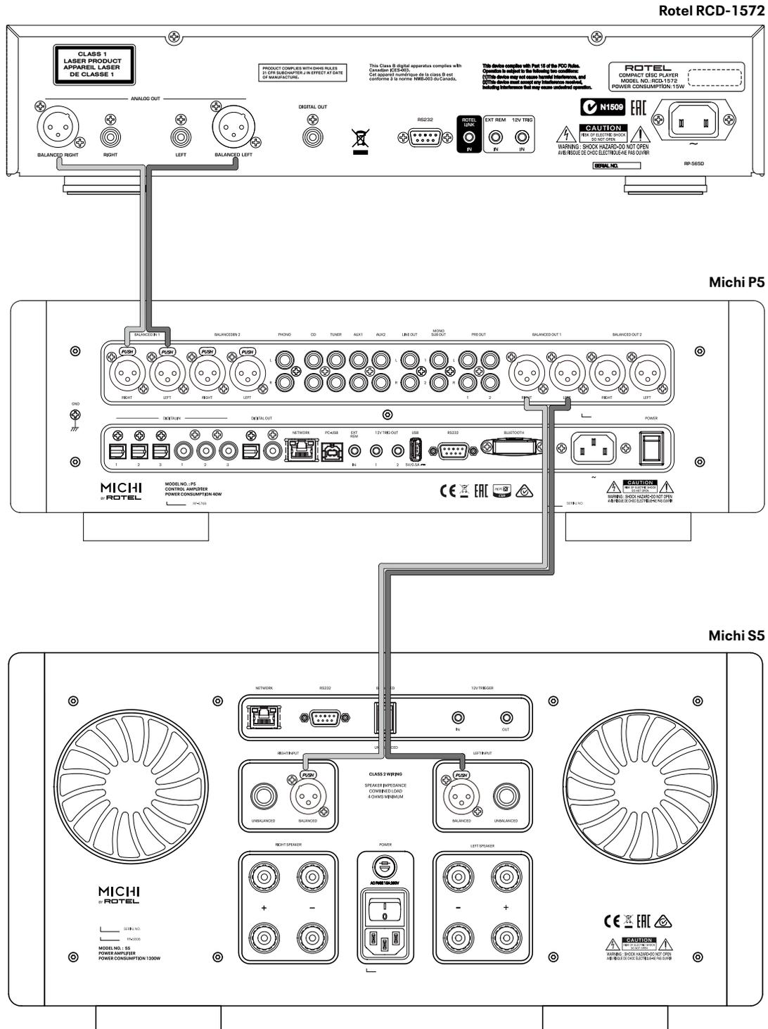
**Figure 5: Digital Inputs and 12V Trigger Output**
