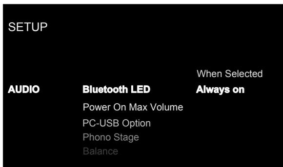
This Audio menu in the Setup menu, provides the following options, selected by placing the highlight on the desired line using the  $\wedge/\vee$  **(D)** arrow buttons and pressing the Enter **(K)** button. This action displays the right side options allowing changes. Change the options using the  $\wedge/\vee$  **(D)** arrow buttons and press the Enter **(K)** button to confirm.
