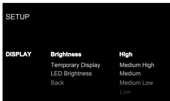
This Display menu in the Setup menu, provides the following options, selected by placing the highlight on the desired line using the  $\wedge/\vee$  **(D)** arrow buttons and pressing the Enter **(K)** button. This action displays the right side options allowing changes. Change the options using the  $\wedge/\vee$  **(D)** arrow buttons and press the Enter **(K)** button to confirm.
