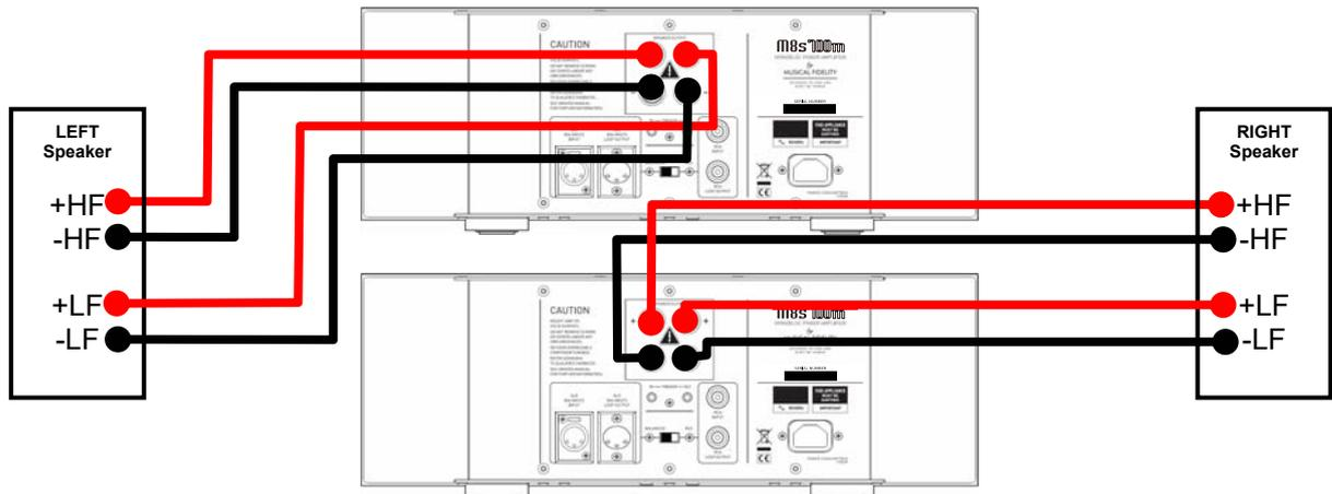
**Bi-wiring speaker leads connection diagram.**
