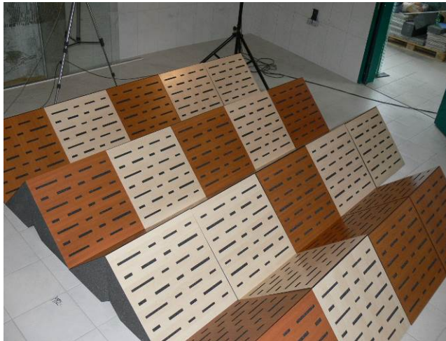
Picture 5: test samples in the reverberation room.
