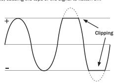
When the 851W detects clipping this LED will briefly flash. If the clipping reaches a dangerous amount that could damage the amplifier or attached speakers the unit will then go into protection.
