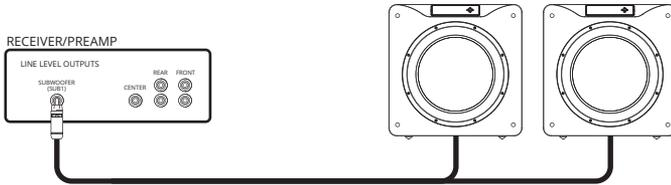
Another option is to use the Left and Right RCA or XLR outputs on the SB16-Ultra to Daisy Chain additional subwoofers. It's important to use the matching output and input terminals. For example, if you are using the RCA inputs, be sure to use the RCA outputs to daisy chain to the next subwoofer.
