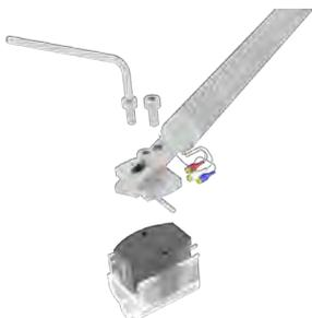
Now you can connect the respective signal cable with the matching color pins of the cartridge.
