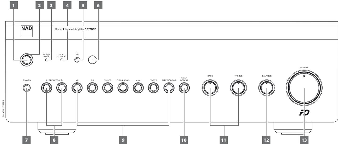
**1 STANDBY:** With the rear panel POWER switch set to ON position, press this button to switch ON the C 375BEE from standby mode. The Standby LED indicator will turn from amber to blue. Pressing the STANDBY button again turns the unit back to standby mode.
