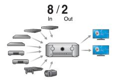
This unit is equipped with 8 HDMI inputs and 2 HDMI outputs enabling connection to various HDMI compatible devices such as Blu-ray Disc players, game consoles and HD video camcorders. This unit is equipped with 2 monitor outputs, enabling you to project the same image at the same time using this unit.
