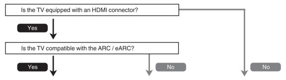
"Connection 1: TV equipped with an HDMI connector and compatible with the ARC (Audio Return Channel) / eARC (Enhanced Audio Return Channel)" (FF p. 53)
