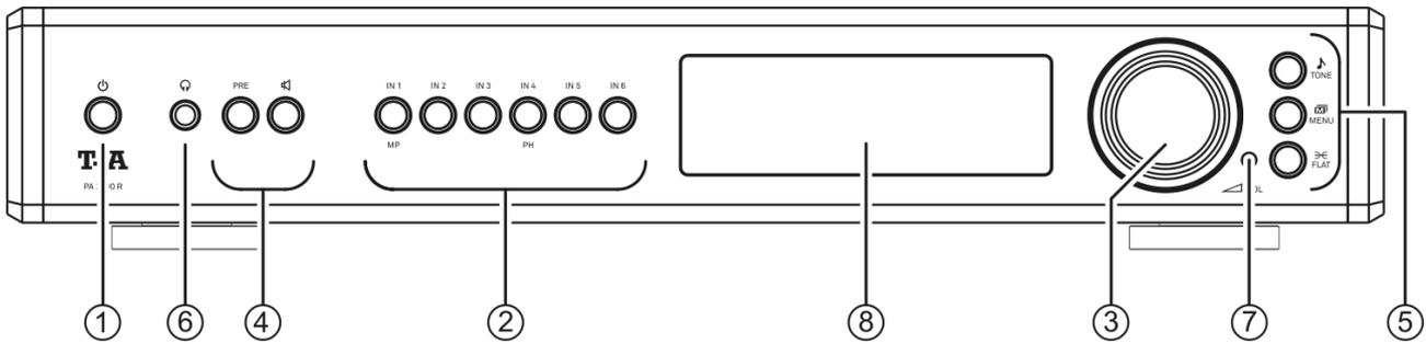
All the important functions of the **PA 2000 R** can be controlled using the buttons and rotary knob on the front panel. Direct-acting buttons are provided for fundamental functions such as source selection. Functions which are needed less frequently are controlled using menus which are called up by pressing the **MENU** / **TONE** button.
