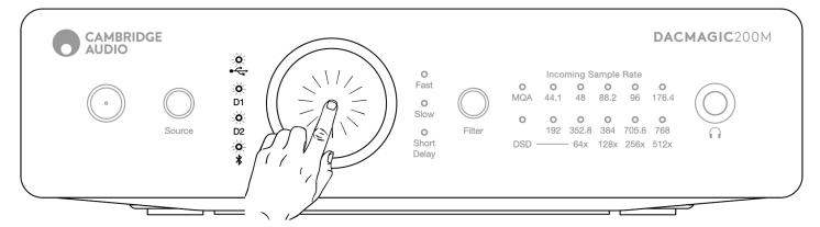
APD OFF - Press and hold down the Volume knob for 5 seconds, and wait for the Input LEDs to blink 2 times.
