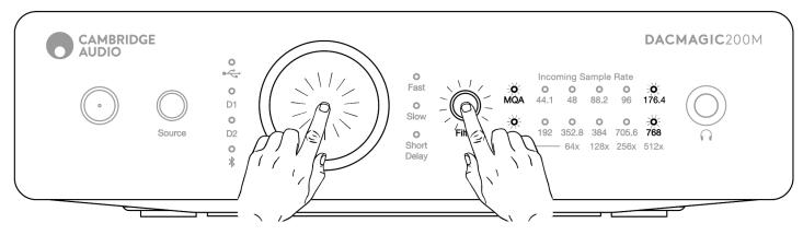
Fixed/variable out mode is toggled by short pressing the Volume knob and the Filter button at the same time:
