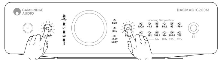
Short press both Source and Filter buttons. All LEDs will light in sequence, one by one.
