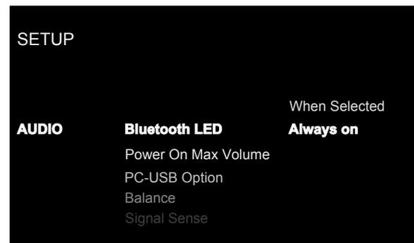
This Audio menu in the Setup menu, provides the following options, selected by placing the highlight on the desired line using the ^/∨ (D) arrow buttons and pressing the Enter (K) button. This action displays the right side options allowing changes. Change the options using the ^/∨ (D) arrow buttons and press the Enter (K) button to confirm.
