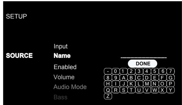
1. Press the ^/∨ (D) arrow buttons on the remote control to change the first letter, scrolling through the list of available characters.
