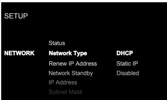
This Network menu in the Setup menu, provides the following options, selected by placing the highlight on the desired line using the ^/∨ (D) arrow buttons and pressing the Enter (K) button. This action displays the right side options allowing changes. Change the options using the ^/∨ (D) buttons and press the Enter (K) button to confirm.
