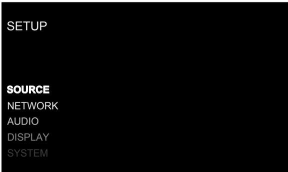
The Setup menu provides access to OSD screens for various configuration options. Setup menu is reached by pressing the SETUP (B) button on the remote. To select the desired menu, move the highlight using the ^/∨ (D) arrow buttons and press the Enter (K) button on the remote control. Press the SETUP (B) button again to return to the previous menu or select "EXIT" on the OSD to end setup and return to normal operation.
