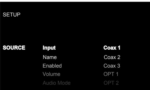
A key step in setting up the unit, is to configure each source input using the Source Setup screens. Configuring the inputs allows you to set defaults for a number of settings including the type of input connector, the desired audio mode, custom labels that appear in the displays when a source is selected, and many more options.
