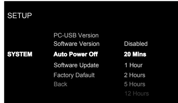
This System menu in the Setup menu, provides the following options, selected by placing the highlight on the desired line using the ^/∨ (D) arrow buttons and pressing the Enter (K) button. This action displays the right side options allowing changes. Change the options using the ^/∨ (D) arrow buttons and press the Enter (K) button to confirm.
