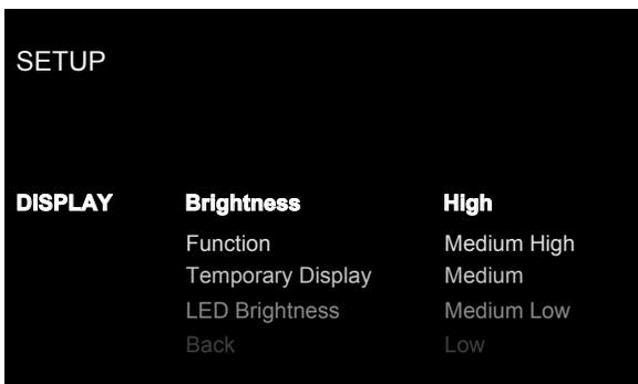
This Display menu in the Setup menu, provides the following options, selected by placing the highlight on the desired line using the ^/∨ (D) arrow buttons and pressing the Enter (K) button. This action displays the right side options allowing changes. Change the options using the ^/∨ (D) arrow buttons and press the Enter (K) button to confirm.
