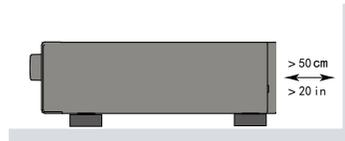
**WARNING:** The rear panel power cord connector is the mains power disconnect device. The device must be located in an open area that allows access to the cord connector.
