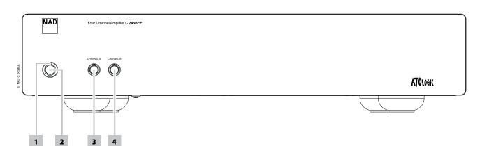
1 **STANDBY BUTTON:** Press this button to switch ON the C 245BEE. The Standby LED indicator will turn from amber to blue. Pressing the STANDBY button again turns the unit back to standby mode.
