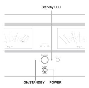
**1** Press ON/STANDBY to set the power amplifier to Standby.
