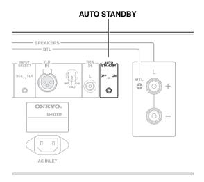
When **AUTO STANDBY** is turned **ON** side, the power amplifier will automatically enter Standby mode if the power amplifier receives no signal for 3 hours.
