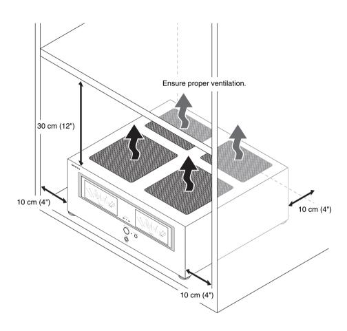
Install the power amplifier on a sturdy rack or shelf. Position it so that its weight is evenly dispersed on its four legs. Do not install the power amplifier in a place with vibration or an unstable location. The power amplifier is designed to have high conversion efficiency, however, its temperature will become much higher than other audio equipment. Therefore, make sure not to hamper heat dissipation by ensuring proper ventilation.
