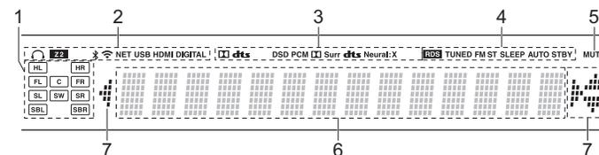
1. Speaker/Channel display: Displays the output channel that corresponds to the selected listening mode.
