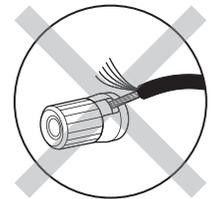
Make sure the exposed wires of the speakers do not stick out of the speaker terminals when connecting. If the exposed wires of the speakers touch the rear panel or the + and - wires touch each other, the protection circuit will be activated.
