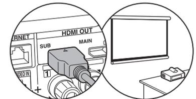
Another TV or projector can be connected to the HDMI OUT SUB jack. This jack does not support ARC. For details about how to output the video to a connected device (→P20)
