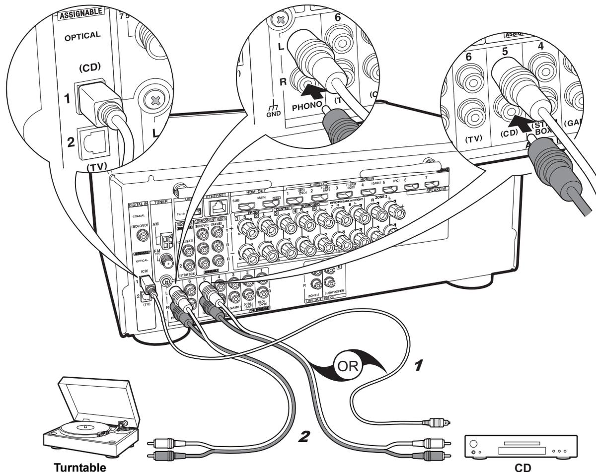
1 Digital optical cable, 2 Analog audio cable
