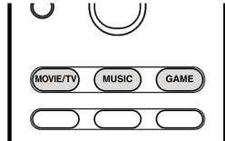
2. Press the selected button repeatedly to switch the modes displayed on the display of the unit.
