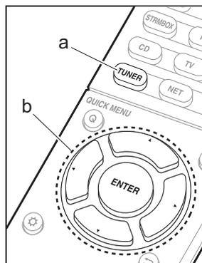
1. Press TUNER (a) on the remote controller repeatedly to select either "AM" or "FM" on the display.
