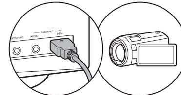
You can connect a device such as a video camera to the AUX INPUT HDMI jack on the front panel.
