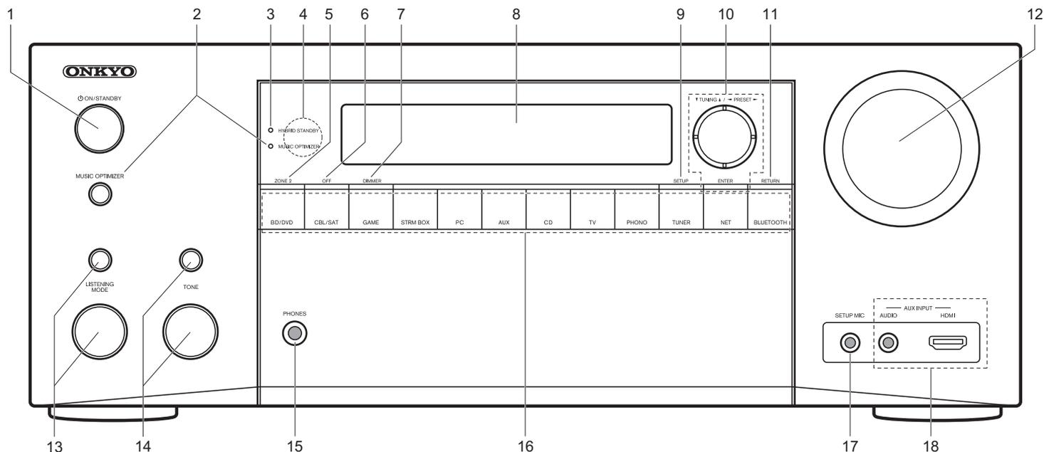
1. **ON/STANDBY** button: Turns the unit on or into standby mode.
