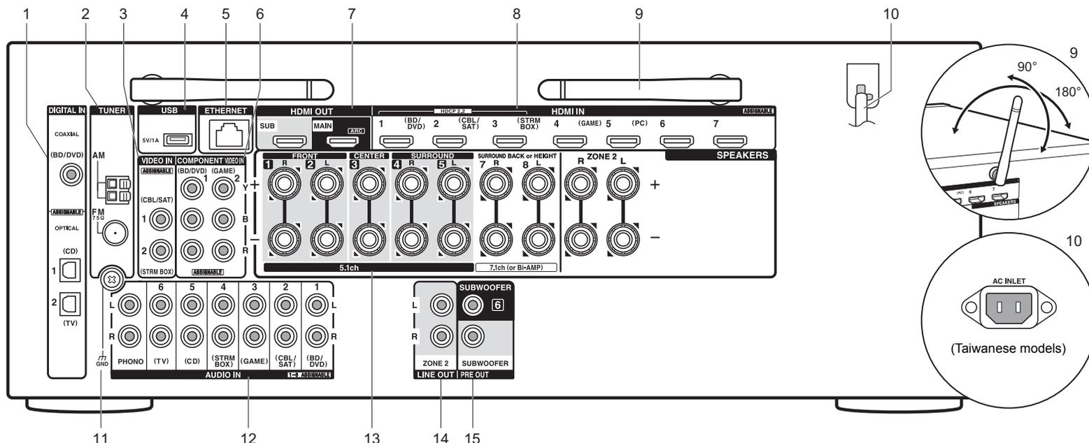
1. DIGITAL IN OPTICAL/COAXIAL jacks: Input TV or AV component digital audio signals with a digital optical cable or digital coaxial cable.
