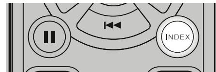
The index system is a method of subdividing tracks into smaller divisions for easier location of those parts. If a disc includes index numbers, playback can be started from any desired index number through the following steps
