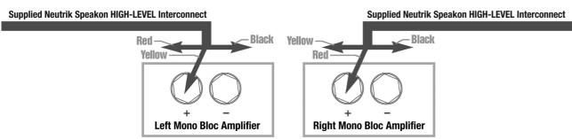
• If connecting a single REL as a dedicated center channel sub, please consider connecting to the rear of the speaker, rather than routing the REL High Level cable all the way back to the amplifier. Connect the black wire of the REL to the negative center channel speaker terminal; twist together the red and yellow wires and connect this pair to the positive center channel speaker terminal.
