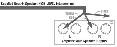
**NOTE:** The SerieT/i models are equipped with internal circuitry to allow seamless connection to Class-D (digital) amplifiers. If connecting to a Class-D amplifier, follow the above connection procedure for differential amplifiers.
