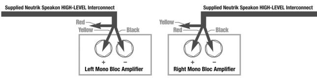
exceptionally high gain (output) from the RELs. If it seems simply too high in gain, please remove either the red or yellow wire from the twisted pair. This will reduce output by half and restore a natural dynamic. If the amplifier is of balanced differential design, please follow the instructions in the section above labeled Differential Connection.
