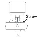
With the aid of a good magnifying glass adjust the needle until it is vertical in the groove (i.e. perpendicular to the record's surface). Ideally this should correspond to the top surface of the cartridge body being parallel to the record surface.
