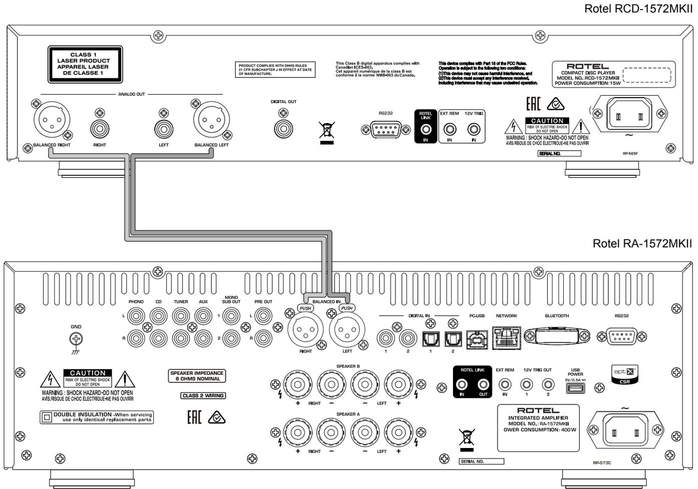
Figure 5 : Digital Output Connection
