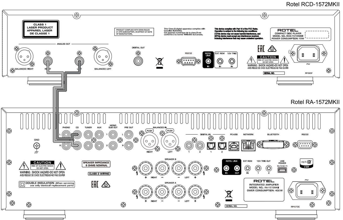
Figure 4 : **Balanced Outputs Connection**
