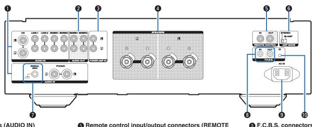
Analog audio input connectors (AUDIO IN) Connecting to a device with analog audio output connectors.
