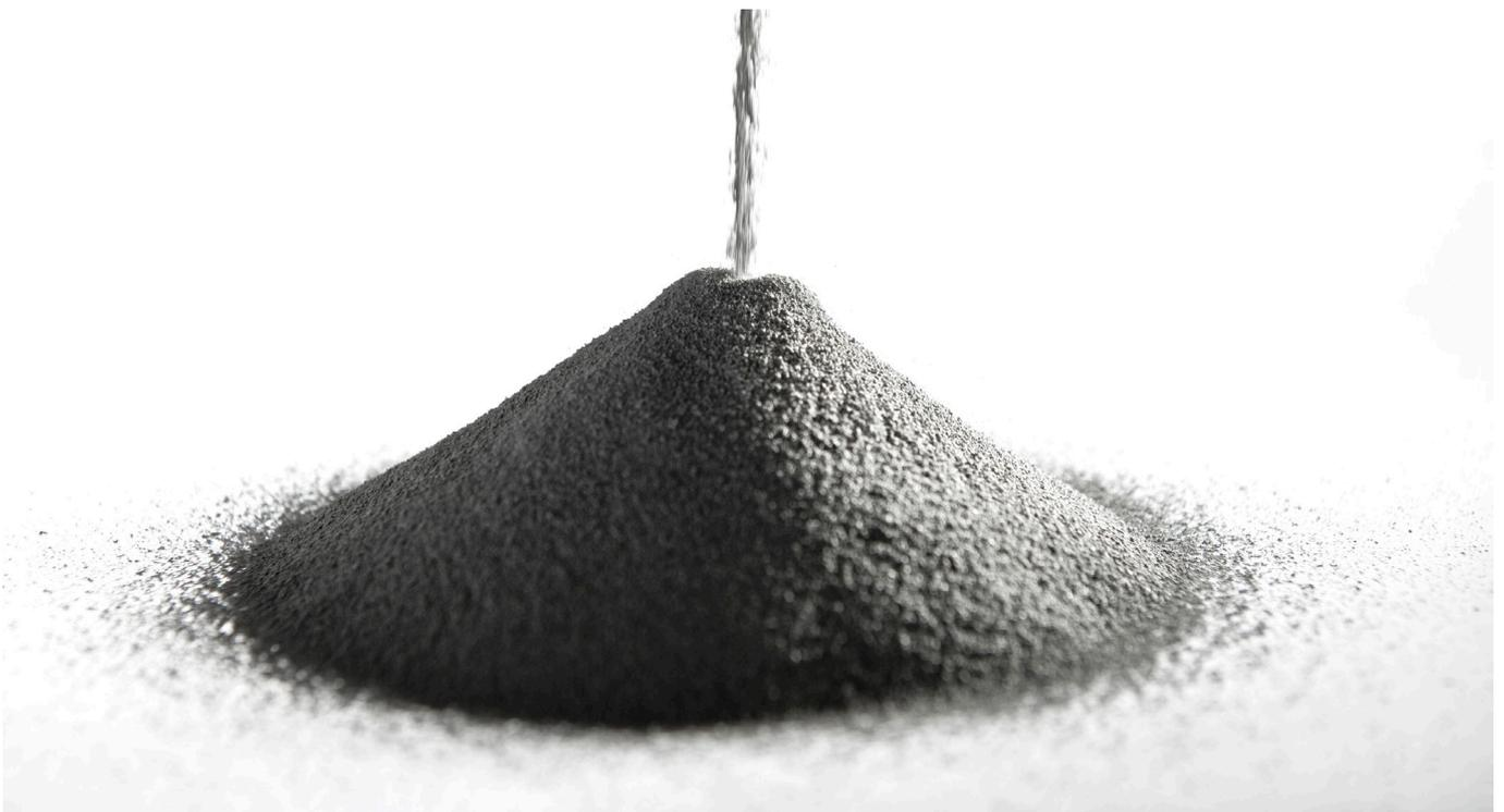
*The individually coated magnet gradual makes it possible to mold a strong magnet that is not electrical conductive.*
