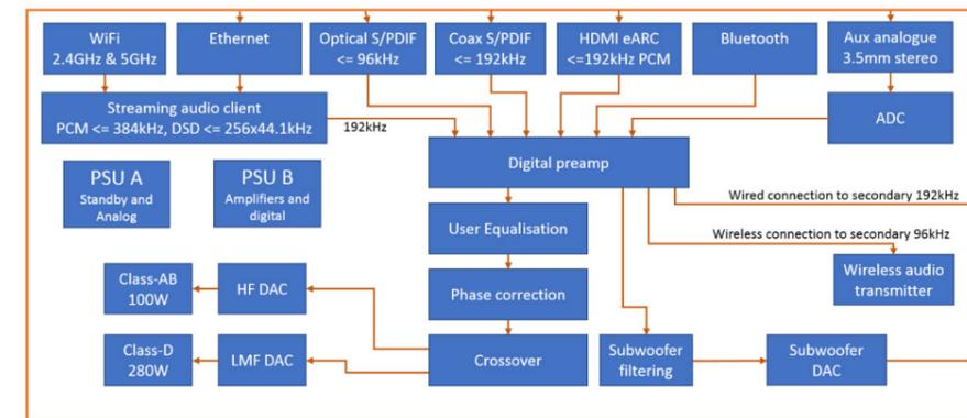
Figure 44 - Block diagram of Primary Electronics
