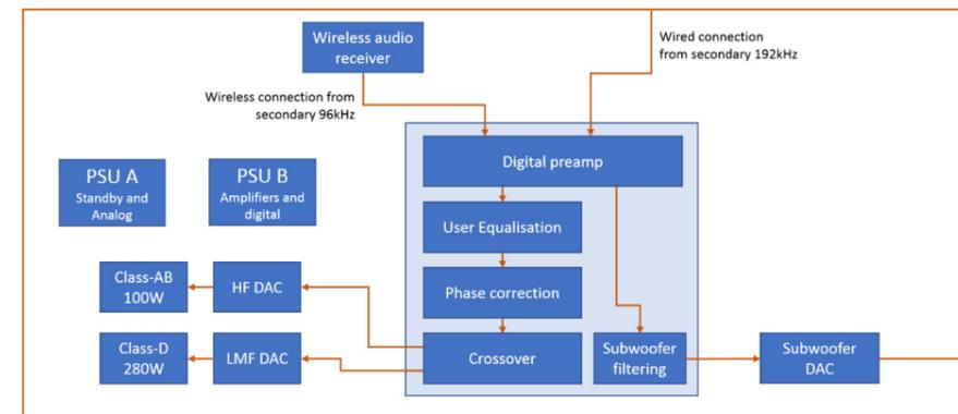
Figure 45 - Block diagram of Secondary Electronics
