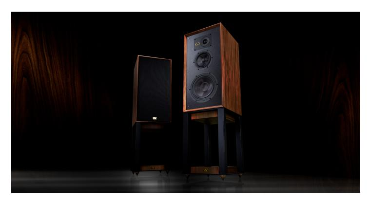
As before, the upgraded cabinet marks the entry of the 'Super' status. Enlarged in volume by increasing the height by 50mm (2 ins), the new cabinet uses a sandwich construction of layers of MDF coupled by latex-based damping glue, specially formulated to reduce panel resonance to below audibility. Pads of thick acoustic damping foam line the cabinet walls, while the interior space is filled with long-hair fibre, both aiding the absorption of internal resonances.
