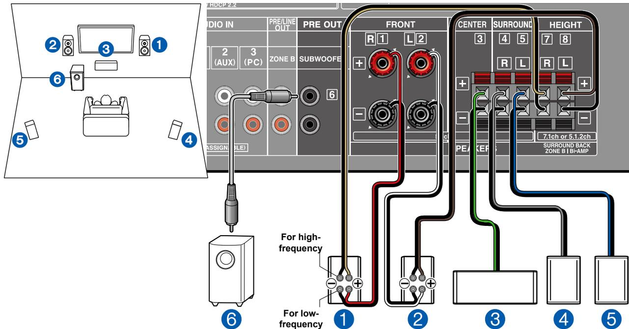
You can configure a 5.1 Channel System ( →p23) by connecting front speakers that support Bi-Amping connection. The Bi-Amping connection can improve the quality of the low and high pitched ranges. Be sure to remove the jumper bar connecting between the woofer jacks and tweeter jacks of the Bi-Amping supported speakers. Refer to the instruction manual of your speakers as well.
