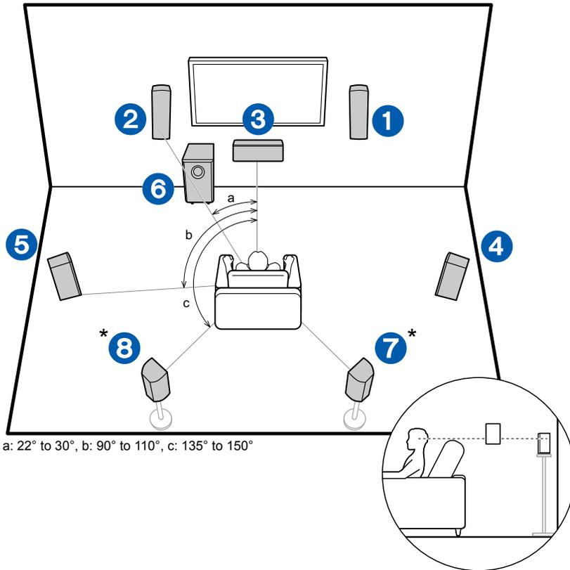
Front speakers output the front stereo sound, and a center speaker outputs the sound of the center of the screen, such as dialogs and vocals. Surround speakers create the back sound field. Powered subwoofer reproduces the bass sound, and creates the rich sound field. Surround back speakers improves the sense of envelopment and connectivity of sound in the back sound field, and provides a more real sound field.
