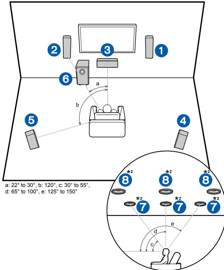
This is a 5.1.2 Channel System that combines the supplied speaker system with separately available top front speakers, top middle speakers, or top rear speakers.
