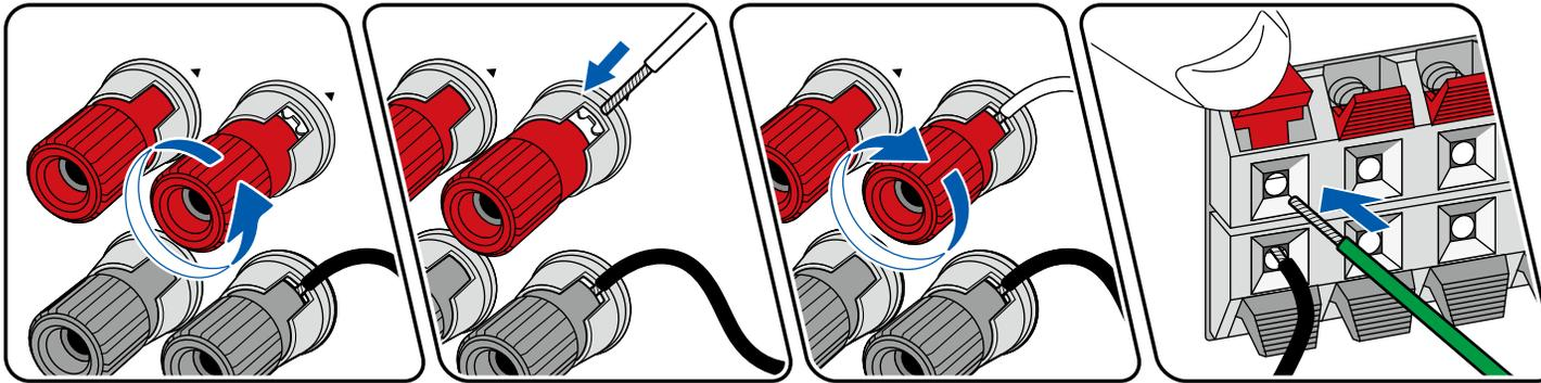
Make correct connection between the unit's jacks and speaker's jacks (+ side to + side, and - side to - side) for each channel. If the connection is wrong, a bass sound will not be reproduced properly due to reverse phase. The wires exposed from the tip of the speaker cable do not stick out of the speaker terminal when connecting. If the exposed wires touch the rear panel, or the + side and - side wires touch each other, a malfunction may occur.
