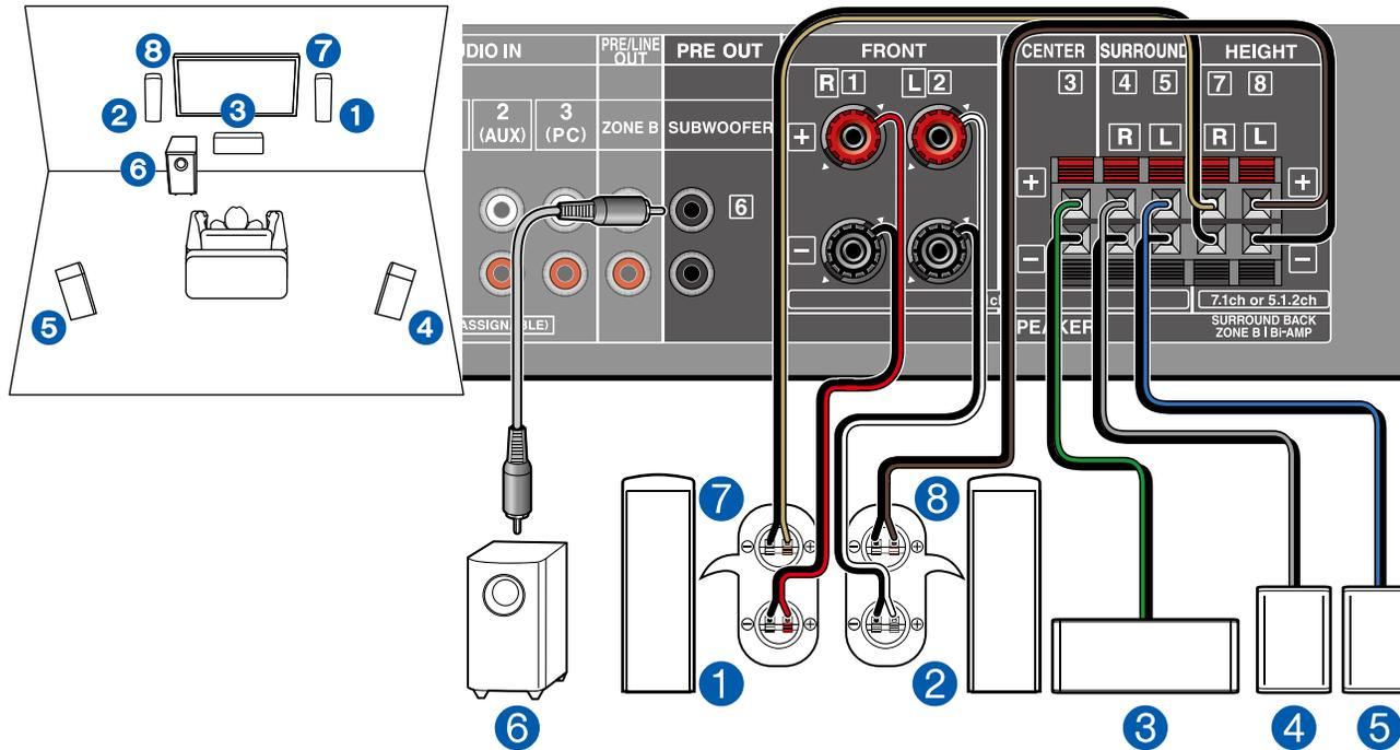
□ Example installation when the entire supplied speaker system is connected (→p26)
