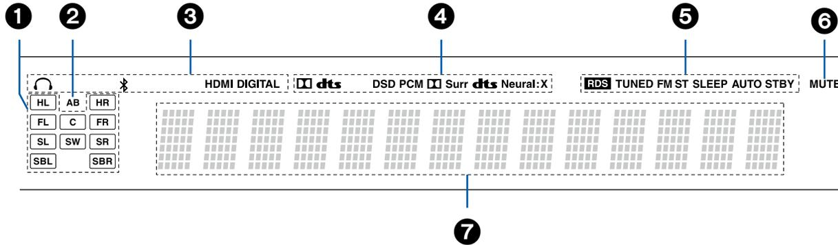
1. Speaker/Channel display: Displays the output channel that corresponds to the selected listening mode.
