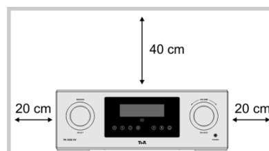
If the system components are to be stacked then the amplifier must be the top unit. Do not place any object on the top cover.
