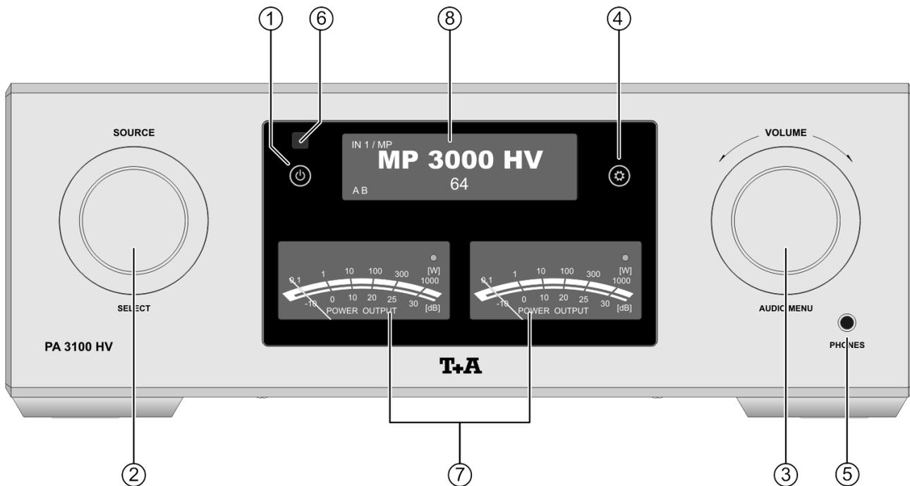
Source selection and volume control are carried out using the large rotary knobs. Functions which are less frequently needed are controlled by means of menus, which are called up using the
