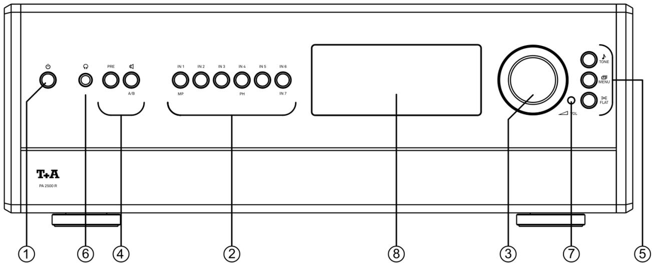
All the important functions of the **PA 2500 R** can be controlled using the buttons and rotary knob on the front panel. Direct-acting buttons are provided for fundamental functions such as source selection. Functions which are needed less frequently are controlled using menus which are called up by pressing the **MENU** / **TONE** button.
