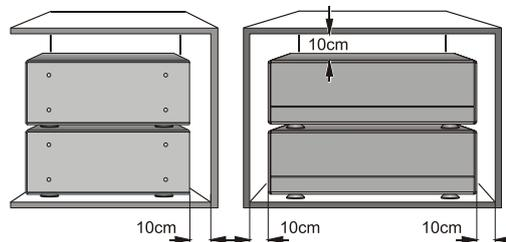
If the system components are to be stacked then the amplifier must be the top unit. Do not place any object on the top cover.
