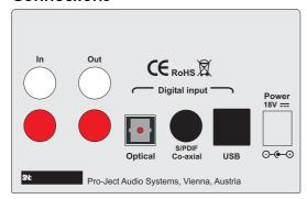
Make all connections, except the connection to the computer and the headphone, whilst the unit is disconnected from the power supply.
