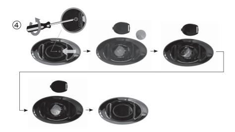
Before first use, loosen the screw (PH00 screwdriver), remove the back cover, remove the battery protection tab, replace the cover, retighten the screw.
