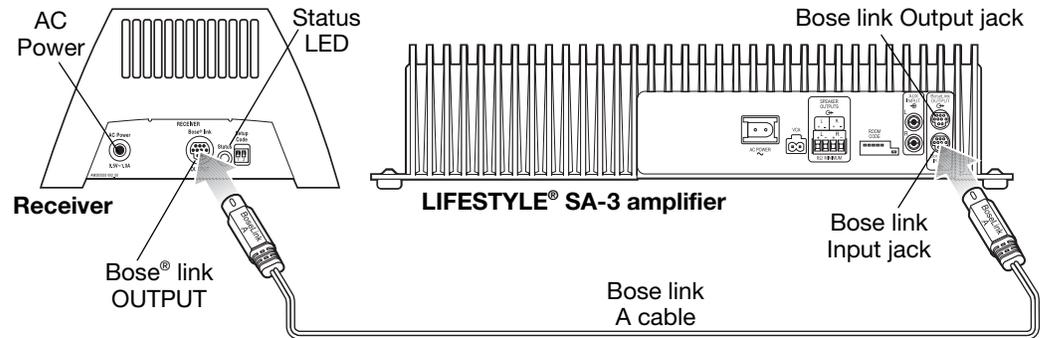
3. Insert the small plug on the power pack cable into the AC Power jack on the receiver and plug the pack into a wall outlet.
