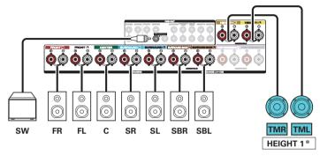
\* The top front or top rear speakers can be connected instead of the top middle speakers. In this case, set the ceiling speakers to be connected under "Height" - "Layout" in the menu. (\*\*\*) 2.254)
