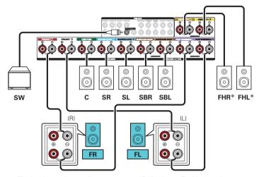
\* The height speakers, ceiling speakers and Dolby Atmos Enabled speakers can be connected to the HEIGHT1 speaker terminals. Set the speaker to be connected from "Height" - "Layout" in the menu. (② p. 254)
