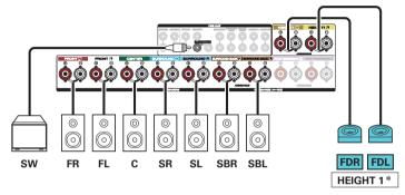
\* The surround Dolby speakers can be connected instead of the front Dolby speakers. In this case, set the Dolby Atmos Enabled speakers to be connected under "Height" - "Layout" in the menu. ( \*\* p. 254)
