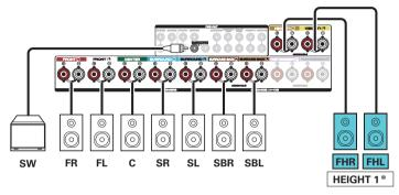
\* The rear height speakers can be connected instead of the front height speakers. In this case, set the height speakers to be connected under "Height" - "Layout" in the menu. (1287 p. 254)
