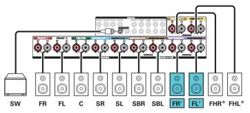
\* The height speakers, ceiling speakers and Dolby Atmos Enabled speakers can be connected to the HEIGHT1 speaker terminals. Set the speaker to be connected from "Height" - "Layout" in the menu. (2 p. 254)
