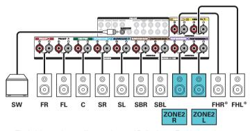
\* The height speakers, ceiling speakers and Dolby Atmos Enabled speakers can be connected to the HEIGHT1 speaker terminals. Set the speaker to be connected from "Height" - "Layout" in the menu. (127 p. 254)
