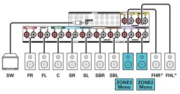
\* The height speakers, ceiling speakers and Dolby Atmos Enabled speakers can be connected to the HEIGHT1 speaker terminals. Set the speaker to be connected from "Height" - "Layout" in the menu. (12 p. 254)
