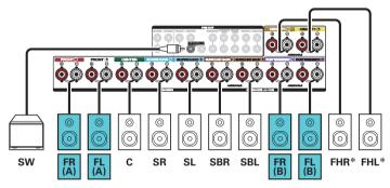
\* The height speakers, ceiling speakers and Dolby Atmos Enabled speakers can be connected to the HEIGHT1 speaker terminals. Set the speaker to be connected from "Height" - "Layout" in the menu. (② p. 254)
