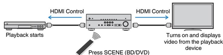
To use HDMI Control, you need to perform the following HDMI Control link setup after connecting the TV and playback devices.
