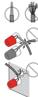
If "Check SP Wires" appear on the front display when the unit is turned on, turn off the unit, and then check the speaker cables short circuit.
