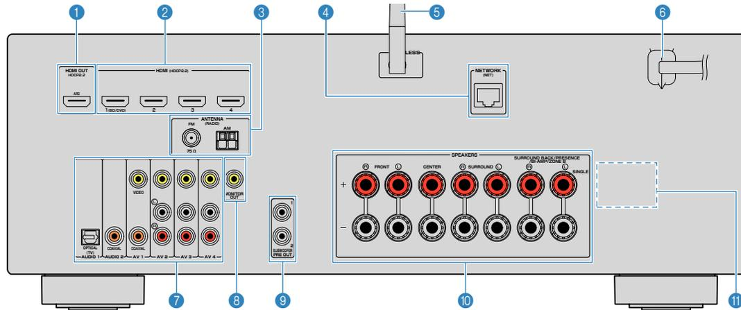
• The area around the video/audio output jacks is marked in white on the actual product to prevent improper connections.
