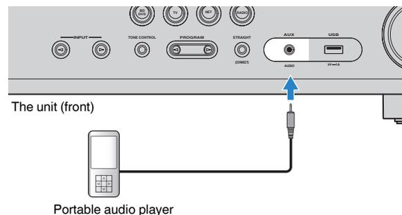
If you select "AUX" as the input source by pressing INPUT, the audio played back on the device will be output from the unit.
