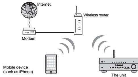
For details on connection, see “Connecting the unit to a wireless network” (p.38).
