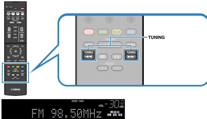
“TUNED” lights up when a signal is received from a radio station.
