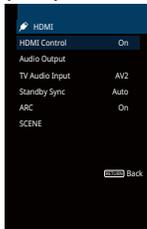
**5** If you made a digital optical cable connection between the TV and the unit, use the cursor keys (Δ/▽) to select “TV Audio Input” and the cursor keys (</>) to select “AUDIO1”.
