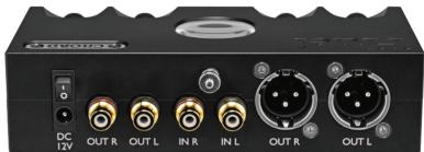
Huei's rear panel carries RCA phono socket inputs only (no balanced XLR). However, output is conveyed by phono sockets and XLR, the latter giving double gain and output. A tiny mains power rocker switch lies here too, just above the 12V d.c. input.
