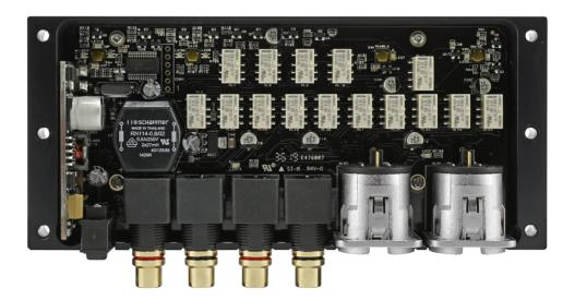
Huei uses a microprocessor (digital!) to select all the many options on offer. Doing so in sensitive low voltage circuits means using high quality sealed miniature relays, seen here as small white rectangles, that click as selections are made. Huei uses miniature surface mount components on a densely populated board; the sockets look vast by comparison.
