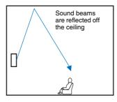
The illustrations above show the path of sound beams when 3D surround is enabled (p. 38) and "Front" in the Channel Out setting is set to "Stereo". (p. 73).
