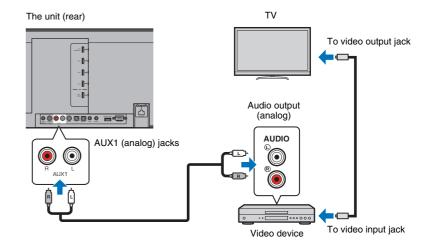
The audio played on the video device will be output though the unit by switching input to AUX1 using the AUX 1 key on the remote control.
