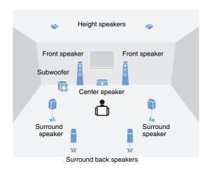
A highly realistic sound field can be created with multiple speakers installed around the listening position as shown in the illustration above. However, this can be difficult to do in a living room. The unit utilizes "digital sound projector" technology, enabling it alone to provide a realistic and engaging surround sound experience.
