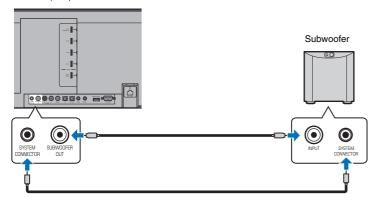
When the unit is connected to the subwoofer via the cable, set the subwoofer output to "Wired" in the setup menu (p. 74)
