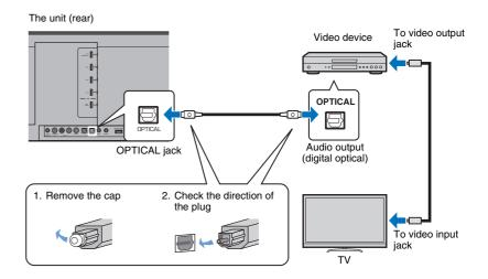
The audio played on the video device will be output though the unit by switching input to OPTICAL using the OPTICAL key on the remote control.
