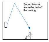
Sound beam output varies depending upon the 3D surround/Surround setting (p. 38, 39) and the channel output setting (p. 73). The illustration above shows the path of sound beams when 3D surround is enabled and "Front" in the Channel Out setting is set to "Beam".
