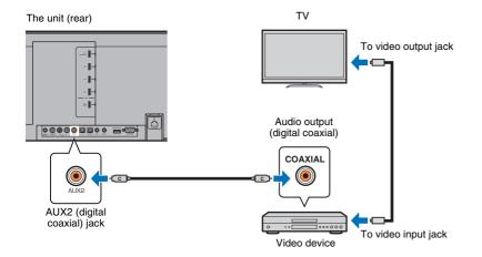
The audio played on the video device will be output though the unit by switching input to AUX2 using the AUX 2 key on the remote control.
