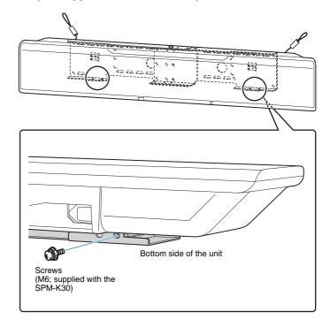
Pass the screws through the loops of the safety wires and then tighten the screws to secure the safety wires to the wall.
