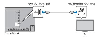
When connecting a TV that supports Audio Return Channel (ARC), enable the HDMI control function (p. 77).
