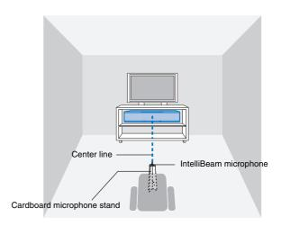
Make sure that there are no obstacles between the IntelliBeam microphone and the walls in your listening room as these objects obstruct the path of sound beams. However, any objects that are in contact with the walls will be regarded as a protruding part of the walls.
