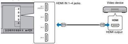
The audio/video played on the video device will be output though the unit by switching input to HDMI 1-4 using the HDMI 1-4 key on the remote control.
