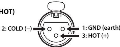
Refer to the instruction manual for the connected component to find out the position of the HOT pin at the balanced output jacks on the component.
