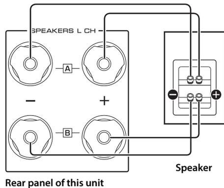
**3 Set the SPEAKERS selector on the front panel to A+B BI-WIRING.**
