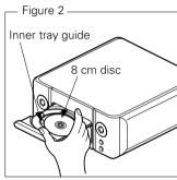
• Place 8 cm discs in the inner tray guide without using an adapter.
