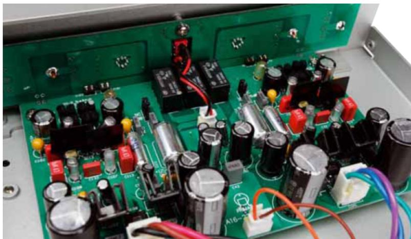
*The board in dual-mono construction located behind the front panel of the Primare*
