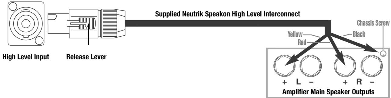
**NOTE:** The REL AirShip II transmitter is equipped with internal circuitry to allow seamless connection to Class-D (digital) main amplifiers. If connecting to a Class-D amplifier, follow the above connection procedure for differential amplifiers.
