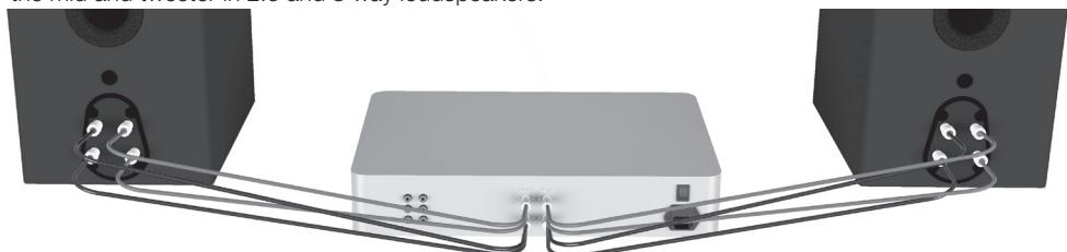
**NOTE: When using this method the terminal links MUST be removed.**
