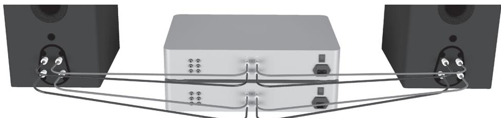
**NOTE: When wiring this method the terminal links MUST be removed.**
