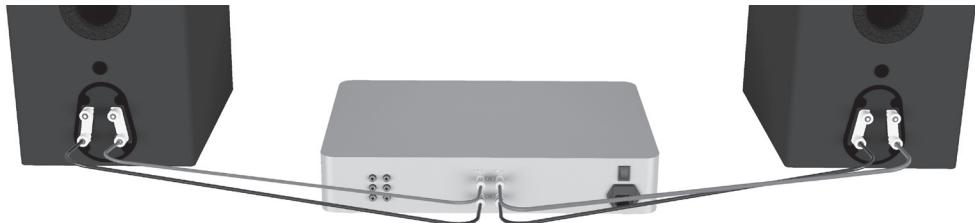
**NOTE: When using this method you must keep the terminal links in place.**
