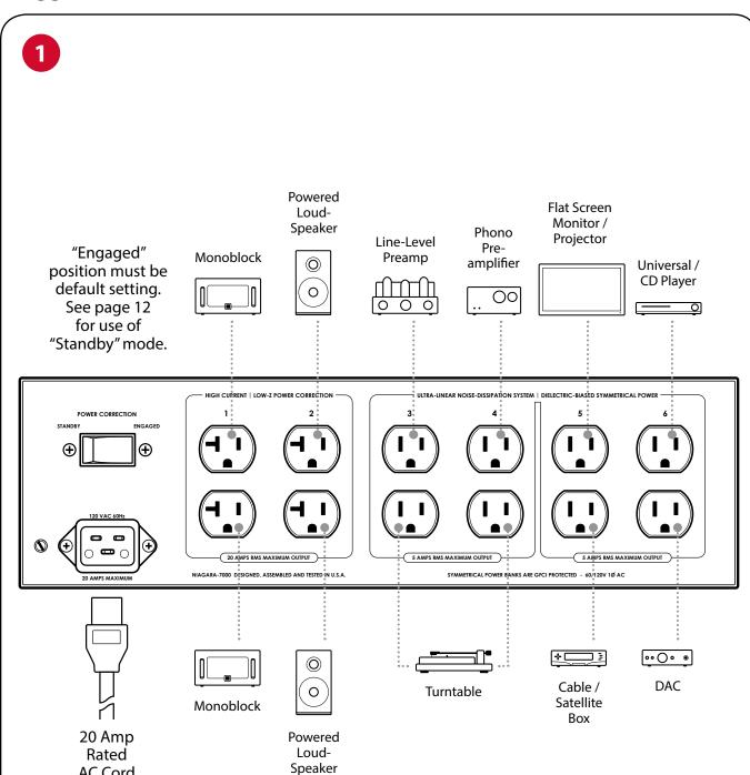
Note: Banks 3 through 6 are subject to many variables and circuit conditions, so experimentation for best results is encouraged. Power amplifiers **must** be connected to banks 1 or 2.
