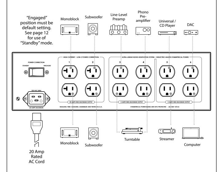
**Note:** Banks 3 through 6 are subject to many variables and circuit conditions, so experimentation for best results is encouraged. Power amplifiers **must** be connected to banks 1 or 2.
