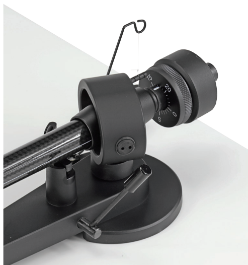
The arm has a damped cue platform with lever, a calibrated rear counterweight and simple weight-end-thread bias that passes over a wire support.
