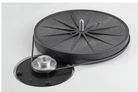
This is the 78rpm belt set up for spinning old shellacs. The large motor pulley diameter is profiled to accept a rubber O ring style belt.
