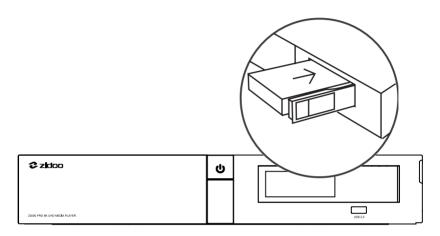
Note: Do not load or replace the hard disk while the device is powered on to avoid damage to the device or hard disk data. Brand new hard disks need to be formatted before loading. This device supports the following hard drive formats: EXT3, EXT4, NTFS, FAT32, EXFAT.
