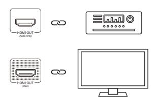
Note: The dual-port output mode is suitable for AV receivers that do not support resolutions higher than 4K or 3D functionality, and when the display device supports resolutions higher than 4K or 3D functionality.
