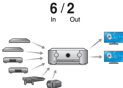
This unit is equipped with 6 HDMI inputs and 2 HDMI outputs enabling connection to various HDMI compatible devices such as Blu-ray Disc players, game consoles and HD video camcorders. This unit is equipped with 2 monitor outputs, enabling you to project the same image at the same time using this unit.
