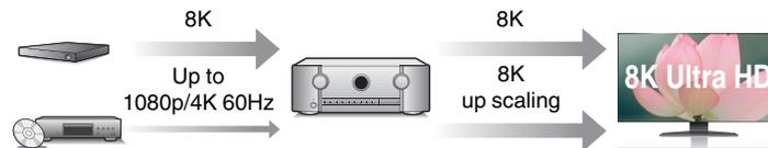
This unit is equipped with a 8K video upscaling function that allows SD (Standard Definition) or HD (High Definition)/4K 60Hz video to be output via HDMI at 8K (7680 × 4320 pixels) resolution. This function enables the device to be connected to a TV using a single HDMI cable, and produces high definition images for any video source.
