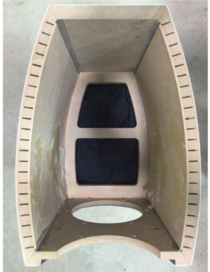
Figure 13: Cross section of Concerta2 F36 baffle showing the Kerf technique.
