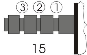
Hang the loop of the thread of the anti-skating weight in the groove of the anti-skating stub (15) corresponding to the downforce applied to your cartridge and hang the thread in the groove of the wire support (17).
