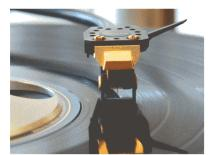
With the stylus guard on and a record on the platter, position the tonearm so that the stylus is over the beginning of the lead out groove. Also adjust the vertical height of The Q UP so that the TONEARM LIFTER it is not touching the tonearm with spacing of about 1.5 mm or 1/16 inch.
