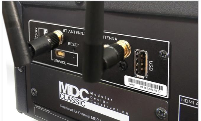
Connect supplied Bluetooth antenna and Wi-Fi antenna\*
