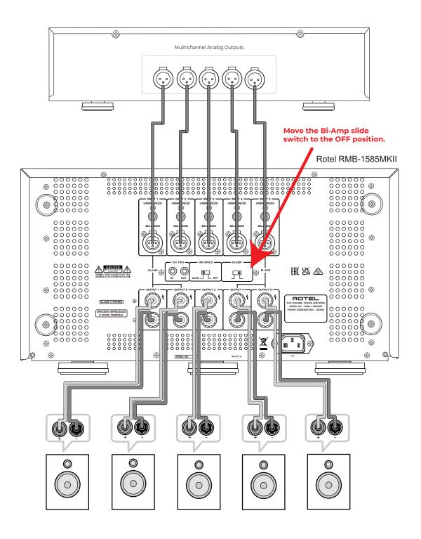
Figure 4: Bi-Amping Connection
