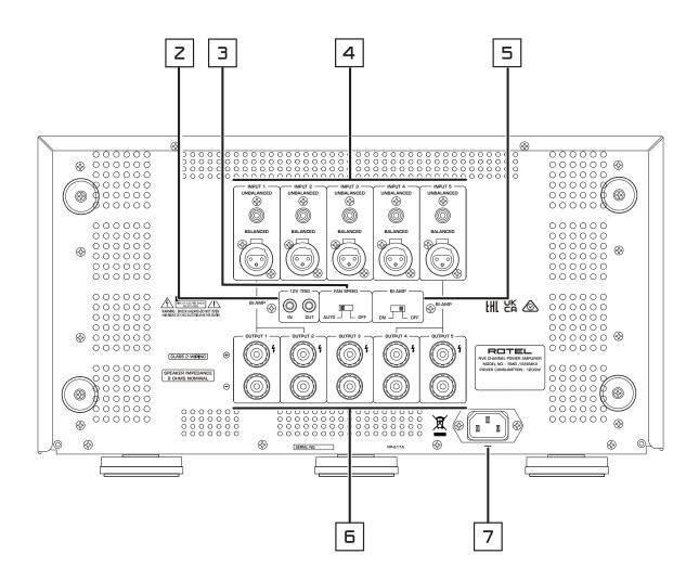
**2**: 12 Volt Trigger Connections Send or receive a 12V trigger signal.
