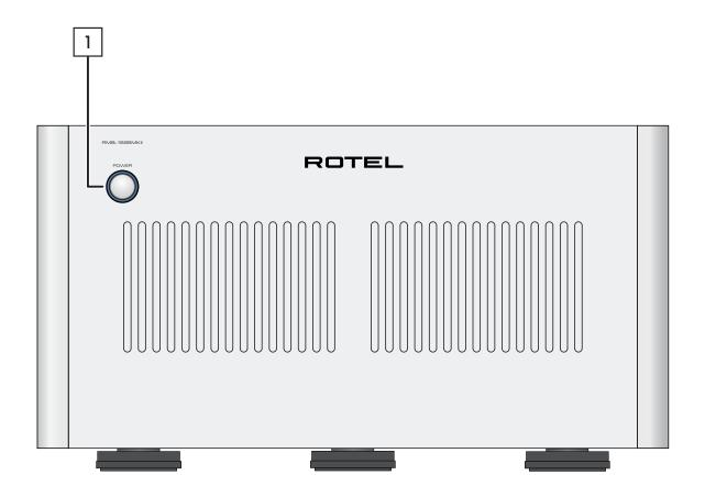
1: Power Button and Power LED Indicator Activate the unit or put it into standby mode.
