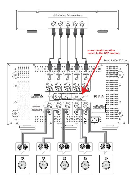
Figure 3: Balanced (XLR) Input Connection
