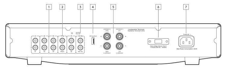
1. Audio inputs (A1-A4) - These inputs are suitable for any 'line level' source equipment such as the audio outputs of CD players, streaming devices such as a Chromecast Audio (RCA Phono to jack cable required) etc.
