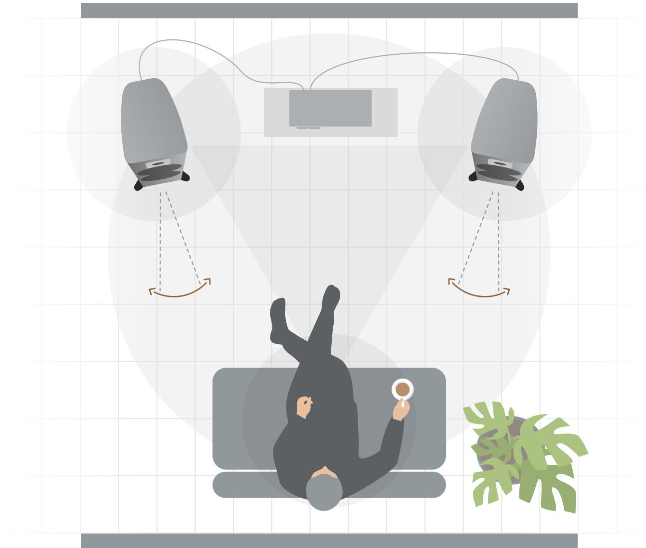
Fig. 5 - Angle loudspeakers inwards to improve imaging.
